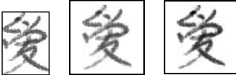
Figure 3: An example image (corresponding to the Chinese character “爱”) after each of the three steps. From left to right: raw input image, resized image, and rescaled image (contrast maximized). Note that black borders are added to the images to show the sizes. The final output with image mean subtracted is not included in this figure.
